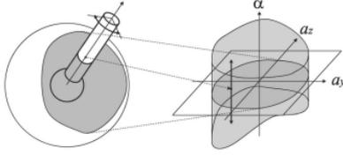
Figure 1: Motion range of a spherical joint projected onto  $(a_y, a_z, \alpha)$  space : [1]
